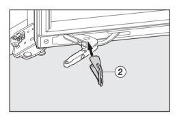
■ Put red restraining clip ② back onto the soft-close mechanism.
